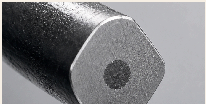
Close-up material surface and steel-core cross section
